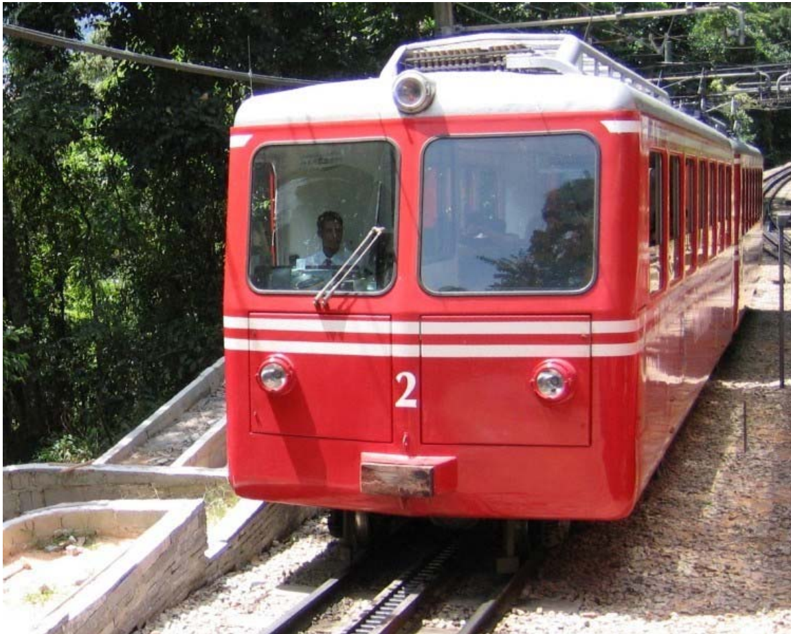
3 phase pantograph on a Corcovado Rack Railway train in Brazil
