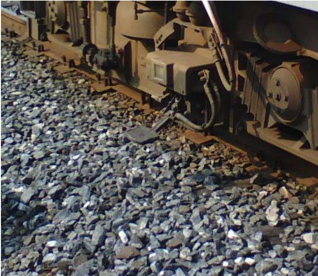
A contact shoe for top-contact third rail on SEPTA's Norristown High Speed Line
