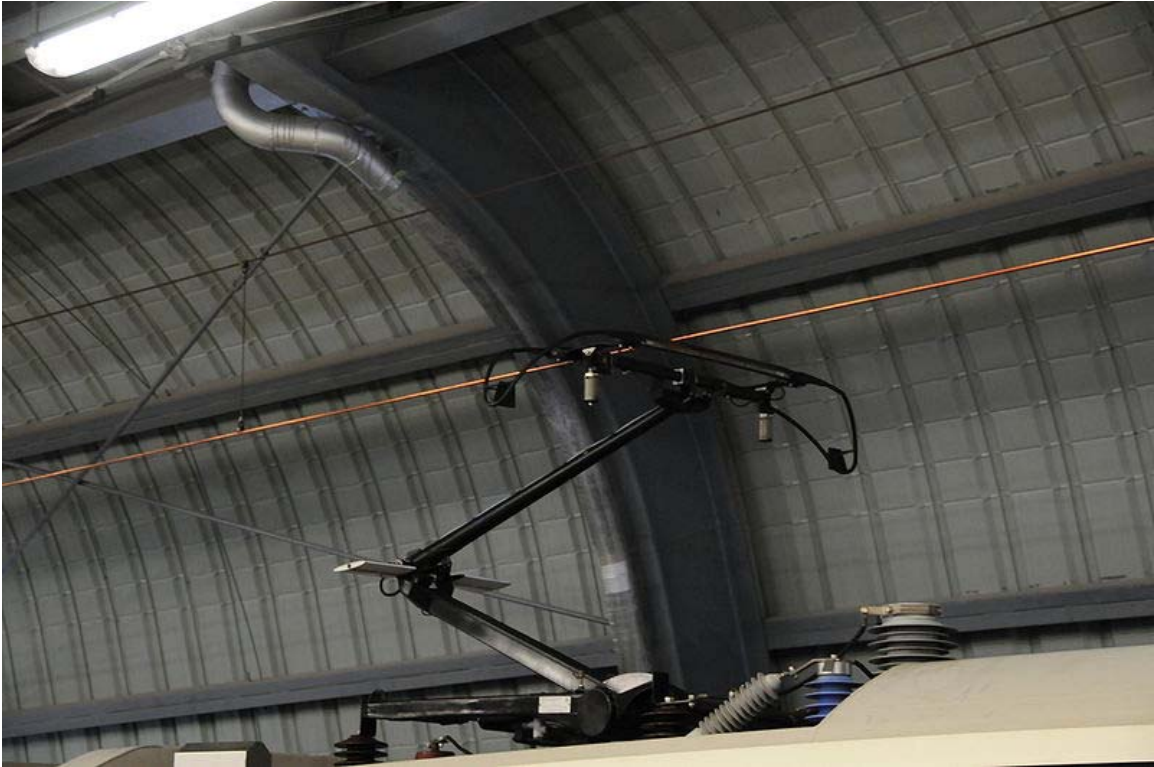
The (asymmetrical) 'Z'-shaped pantograph of the Desiro Class 360/2 EMU on the Suvarnabhumi Airport Rail Link
