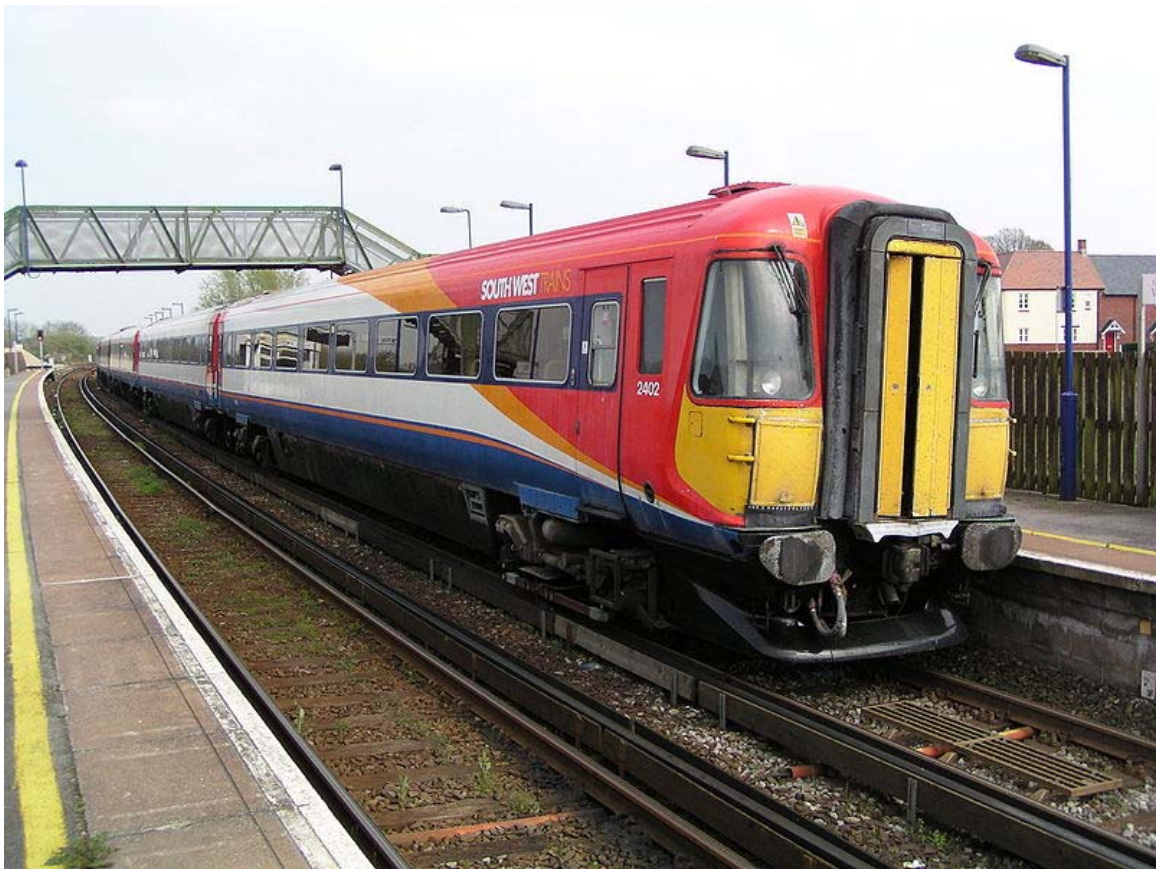
A British Class 442 third-rail electric multiple unit in Dorset. This is the fastest class of third-rail EMU in the world, reaching 108 mph 172 km/h.
