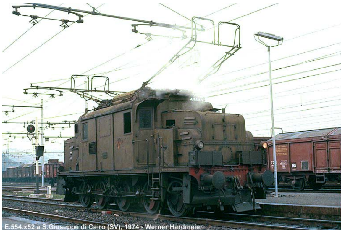
Italian freight locomotive E554 working with three-phase current. Note the two current collectors with separate heads for each phase. Picture taken in Liguria 1974.
