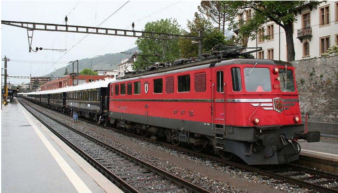
15 kV 16.7 Hz AC traction current used in Switzerland
