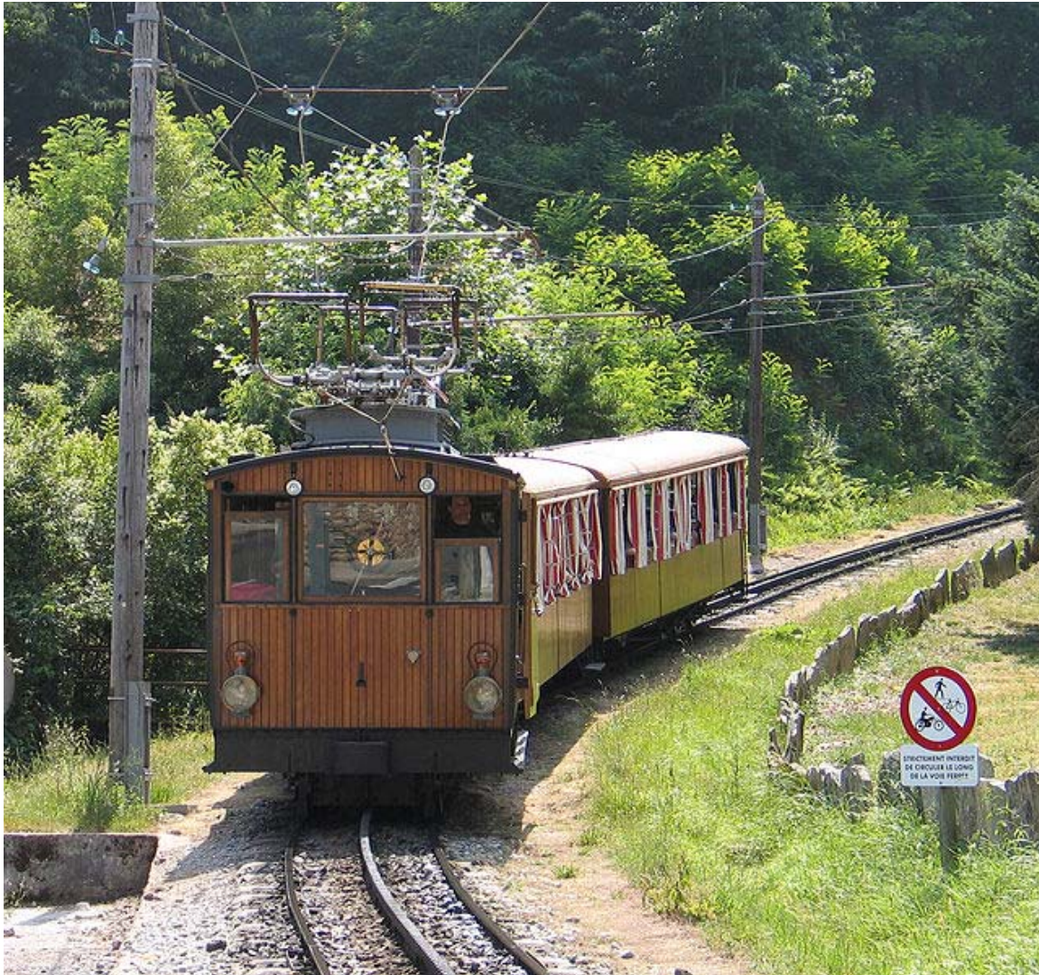
Train using a multiphase electrification system on the Petit train de la Rhune, France
