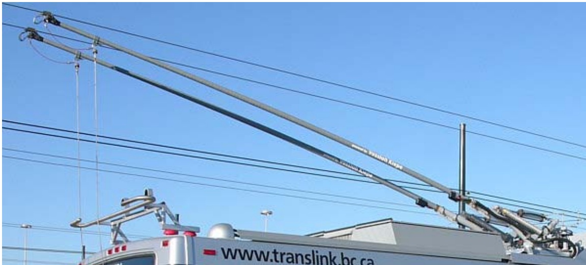
Modern trolley poles as installed on Vancouver's low floor electric trolley buses.
