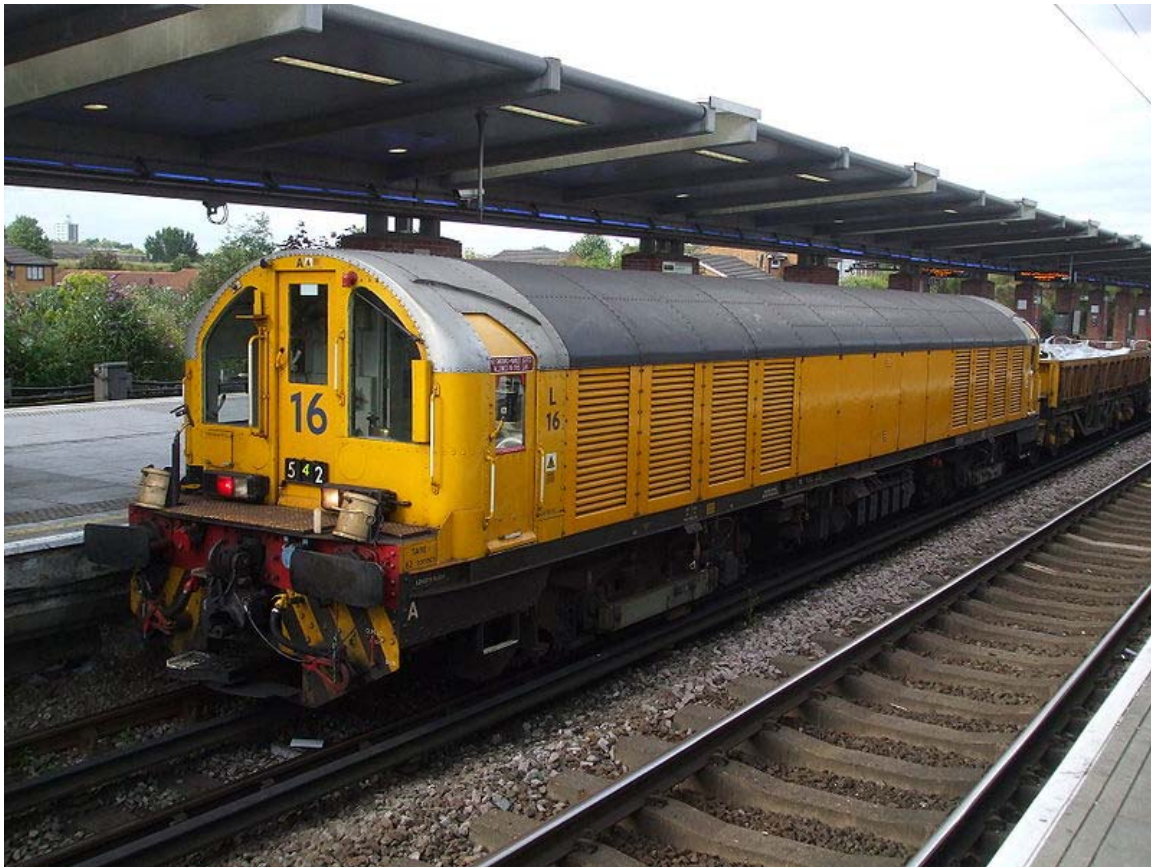
A London Underground battery-electric locomotive at West Ham station
