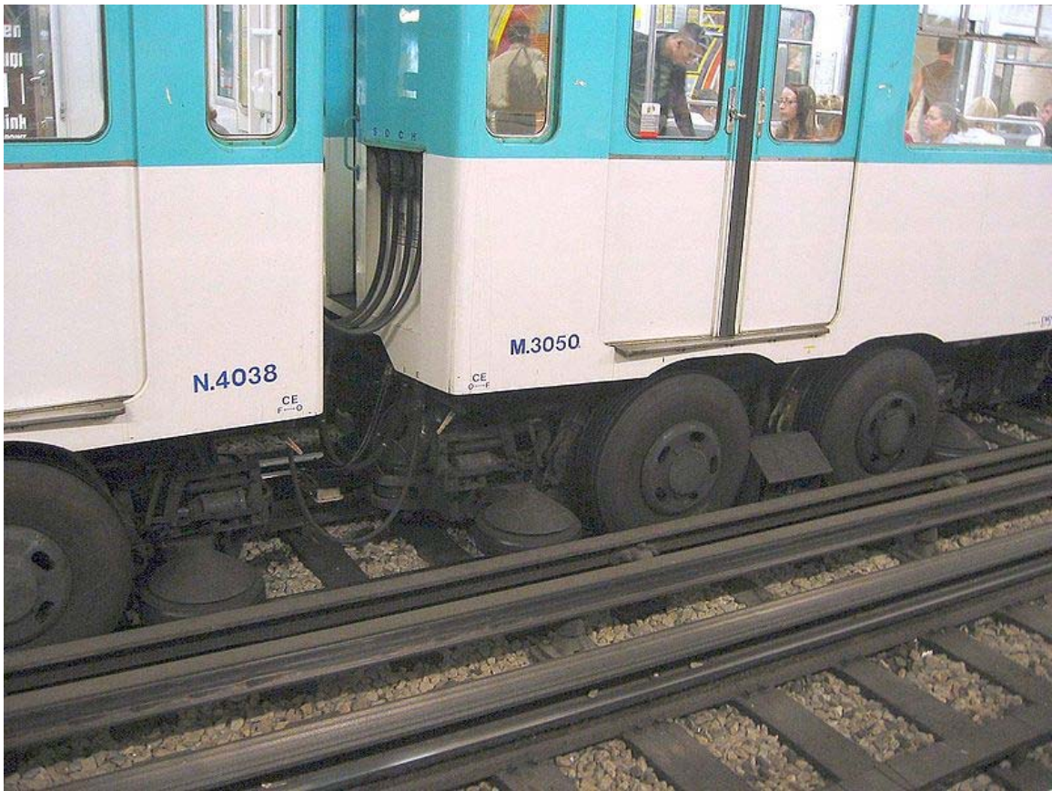
Paris Metro. The guiding rails of the rubber-tired lines are also current conductors. The current collector is between the pair of rubber wheels.
